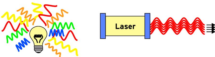
*Fig. 3: The difference between broadband radiation and laser light*
