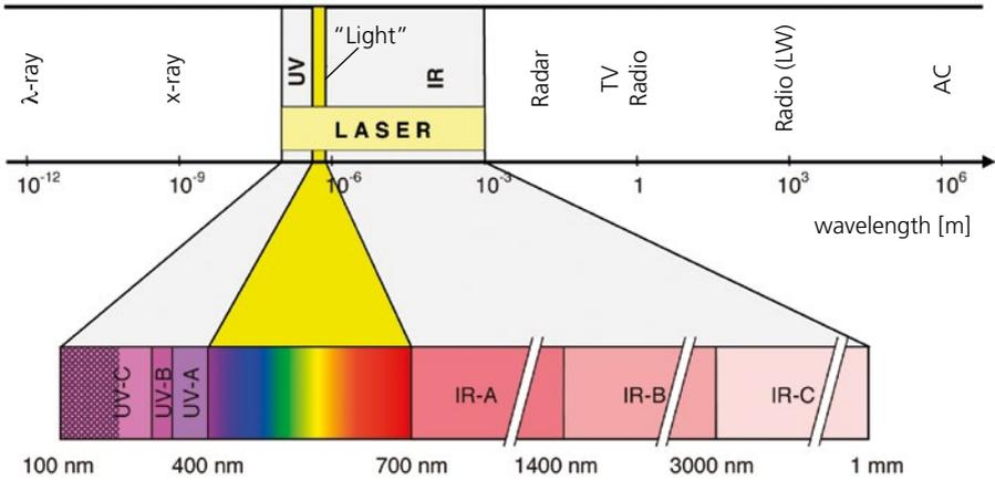
Fig. 2: The electromagnetic spectrum
