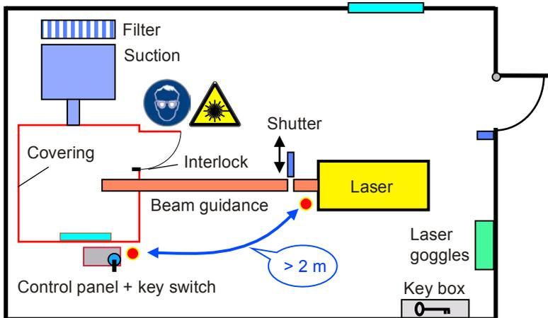
Fig. 21: Labelling and safeguarding of the walk-in process zone as a laser control zone for technical/industrial applications.
