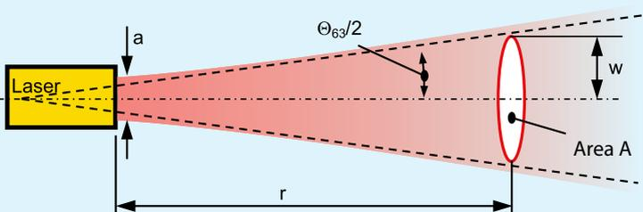
In comparison to the first term in the above equation for  $w$ , the beam radius at the exit aperture of the laser is typically small and can be neglected. Furthermore, for very small angles, the term  $\tan(\Theta/2)$  can be replaced with  $\Theta/2$ .
