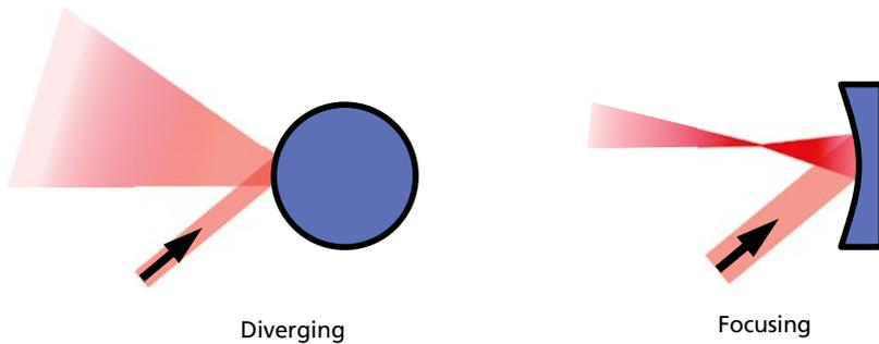
Fig. 9: Focusing and diverging effects of curved surfaces
