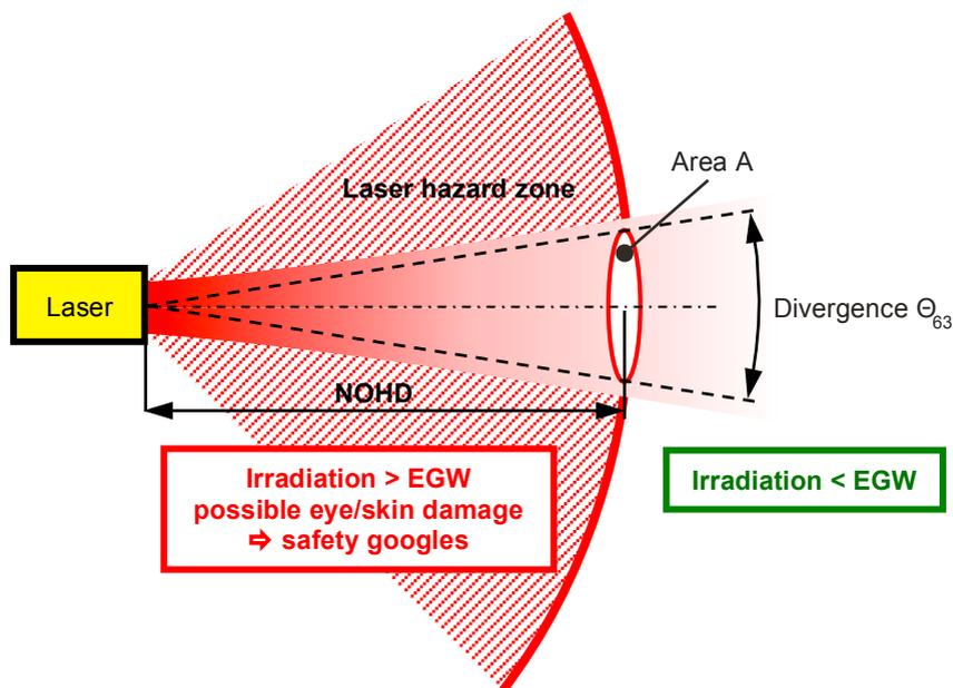
Fig. 17: Laser hazard zone and hazard distance
