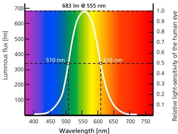
**Fig. A:** Standard spectral sensitivity curve  $V(\lambda)$  for daytime vision pursuant to DIN 5031. For night vision, the curve must be partially moved about 50 nm towards the blue range.
