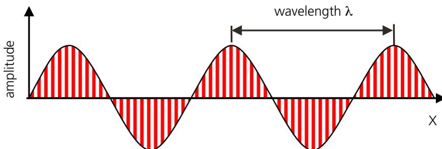
*Fig. 1: An electromagnetic wave is composed of the combination of electric and magnetic waves. Electric waves are used as a reference quantity, which explains why only the sinusoidal electrical wave is plotted in the diagram.*
