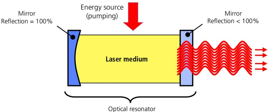
*Fig. 4: Schematic laser design*
