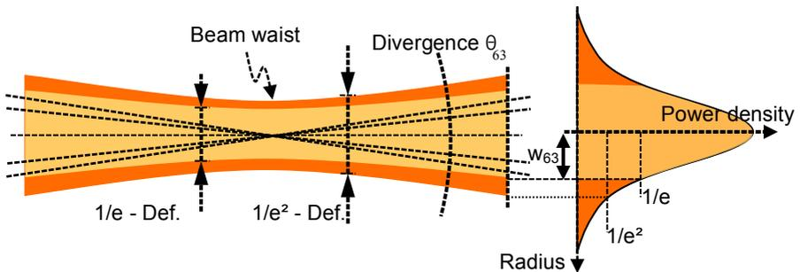
Fig. 11: Radial distribution of power/energy in a Gaussian beam
