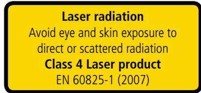
All laser equipment must feature an applied or attached warning text. For laser classes 1 or 1M, reference can be made in the user manual. The sign must include information about the laser class, corresponding warning text, as well as the standards and their publication dates.
