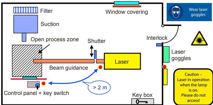
*Fig. 20: The entire room is labelled and safeguarded as a laser control zone for technical/ industrial applications. For medical purposes, the interlock on the door can be omitted.*
